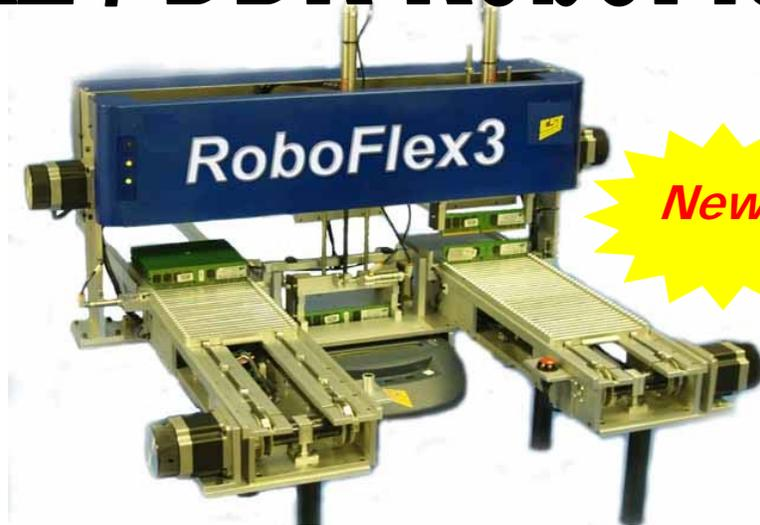
*Pick & Place with DDR2 DIMM Option (Tester not included)*
