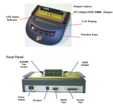
DDR3 1600 MHz DIMM Adapter with a 204pin Stacked Convertor
